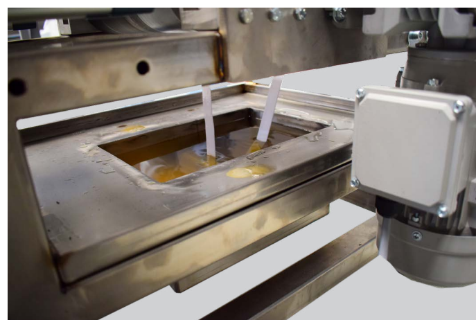
VASCA FOULARD ESTRAIBILE LATERALMENTE FOULARD TUB REMOVABLE LATERALLY
